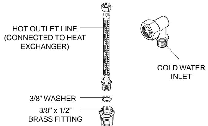
**Fig. 3 - Water connections**
