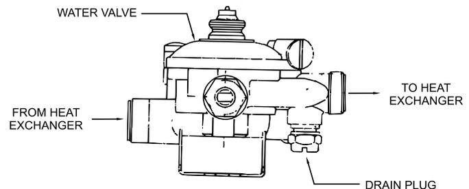
Fig. 0 - Water heater drain plug
