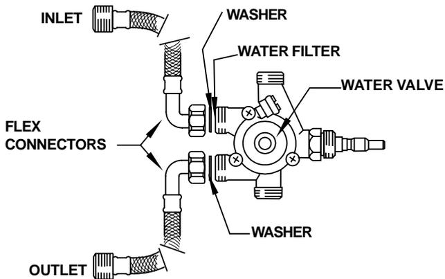
**Fig.7 - Water valve and water connectors, top view**
