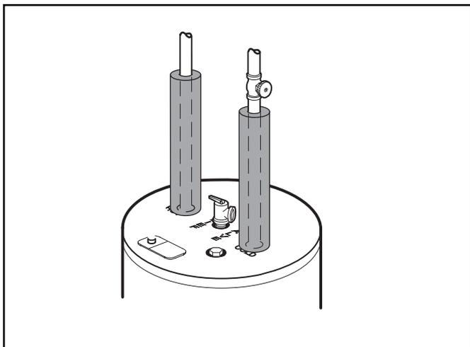
**Figure 1. Typical Vertical piping arrangement.
