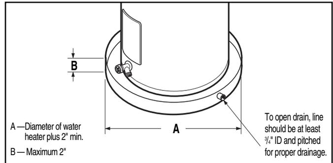
**Figure 1. — Auxiliary Catch Pan**
