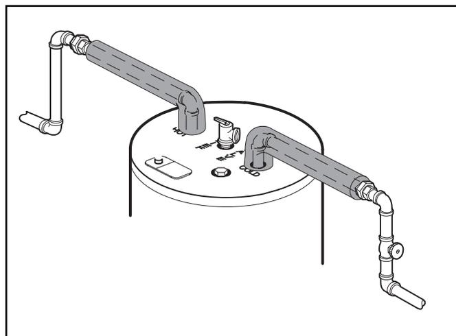
**Figure 2. Typical Horizontal piping arrangement.
