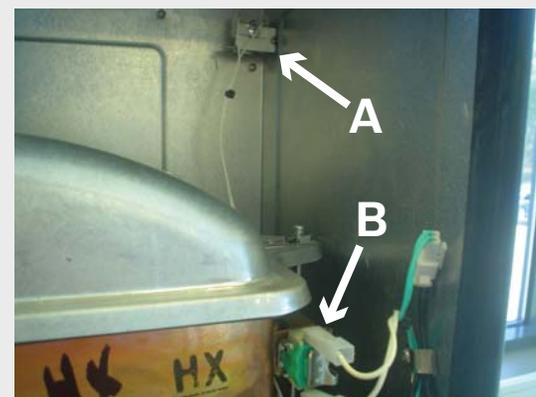
4. Inspect the heat exchanger for signs of exhaust leakage:
