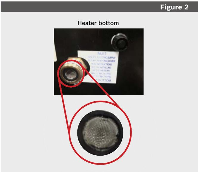
4. Install the inlet screen and attach the water line in accordance with standard plumbing practices. Take care to not get any pipe sealant inside the unit.
